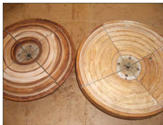
This photo shows the two different sets of jaws I use. On the left is the expanding chuck to hold closed-form bowls from the inside of the rim. On the right is the contracting chuck to hold open-form bowls from the outside of the rim. These are both on Oneway Mega-Jumbo jaws and the diameter closed is 15”.
